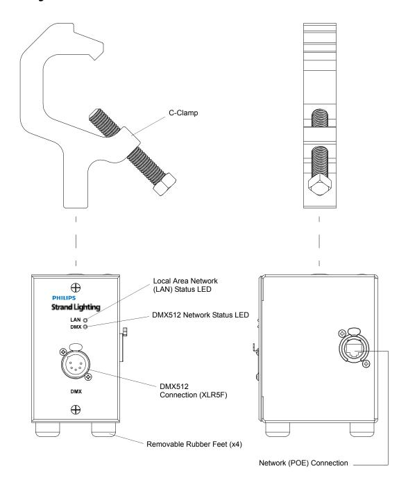
NOTE: Unit can be flush mounted, surface mounted, or hung in truss.
